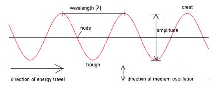
Here we have a representation of transverse waves. We would refer to this as a continuous wave. In the continuous wave are many repeating cycles. A cycle is one complete
