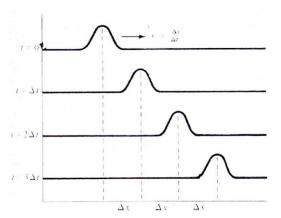
The **speed** of a wave, or in this case a pulse, is computed from the distance it travels and the time required.
