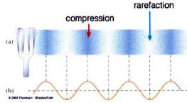
Sound waves are longitudinal waves, sometimes called compressional waves, because when something is vibrating in air, it is alternatingly compressing the air, just as this tuning fork in the diagram.
